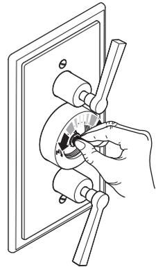
Adjust the cartridge spline whilst measuring the temperature of the water. Ideally the temperature measurement should be taken using a digital thermometer.
