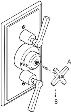
Remove the thermostatic control cross handle/handwheel (A) by unscrewing set screw (B) using a 1.5mm hexagonal key.
