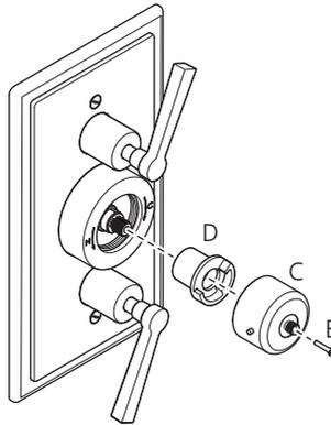
Remove the override (C) and temperature stop (D) by unscrewing and removing screw (E).
