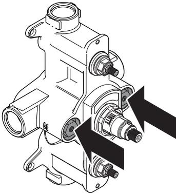
6 Isolate the hot and cold water supplies as follows: The non-return valve covers have a screw in the centre. Use a screwdriver to turn the screws in a clockwise direction until they reach their stop. Do not over tighten the screws as this may damage the non-return valves.
