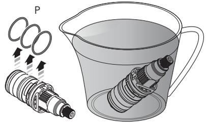
8 Check the 'O' rings (P) for damage (ie. cuts or tears). A set of three replacement 'O' rings are available (PTS027). Remove the 'O' rings before soaking the cartridge in descaling fluid. Soak the cartridge according to the instructions on the descaling fluid packaging. Rinse under cold water before fitting (refer to the 'installing the thermostatic cartridge' section to install).
