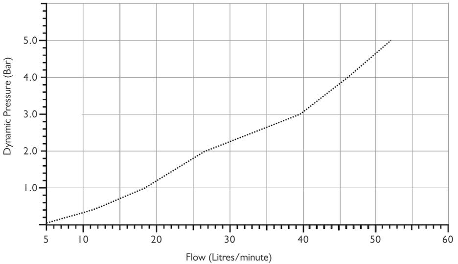
Note: Balanced pressures shown are applied directly to the hot and cold inlets; flow rates indicated are free flowing and may vary subject to restrictions created by installation, pipework, layout or application. Upper and lower outlets have the same flow rates. The outlet temperature during testing was 38°C.
